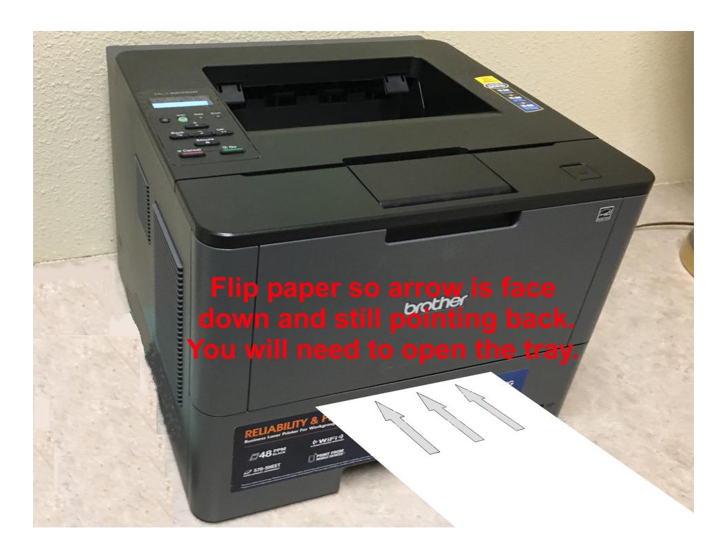
For many printers the input tray is inside a drawer that you pull out and then push closed when ready.
